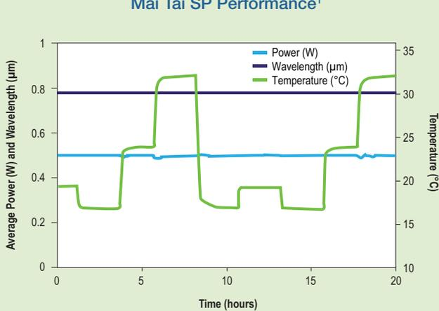
Mai Tai SP performance under  $\pm 8^\circ\text{C}$  temperature swing. Performance values for average power ( $\sim 0.5$  W) and center wavelength stability ( $< 0.3$  nm) are shown.
