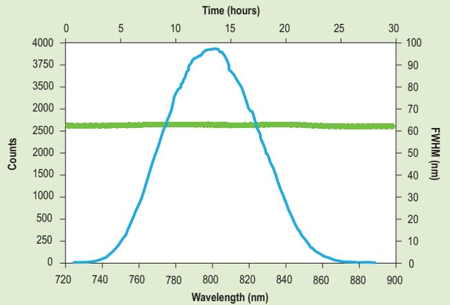
Bandwidth stability of Mai Tai SP over 30 hours (green curve, top and right axes). Typical wavelength spectrum for the Mai Tai SP configured for 60 nm operation (blue curve, bottom and left axes).
