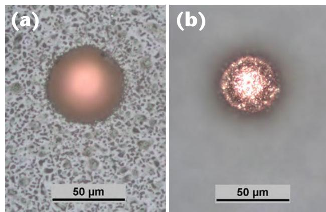
Figure 3: Top ABF surface (a) and bottom copper surface (b) views of a blind microvia drilled with a pulsed UV laser at high PRF with 3,300 holes/sec throughput.
