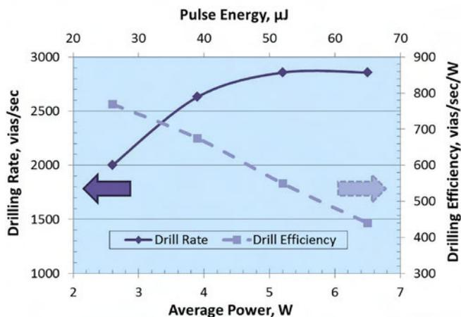
Figure 2: Via drilling rate and efficiency with increasing average power at a fixed PRF. NOTE: This data is at a condition of non-optimized system configuration and process parameter set.
