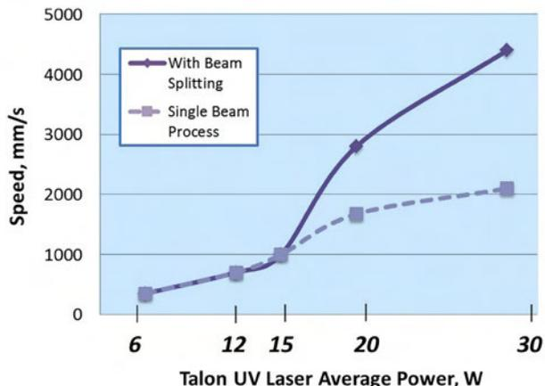
Figure 6: Coverlay patterning—high-speed cutting of thin polyimide, can benefit greatly from a split-beam system configuration.
