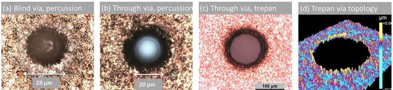
Figure 5: Optical photomicrographs of blind (a) and through (b) vias in Cu/PI/Cu laminate as well as trepanned via (c), and surface topology of trepanned via (d) generated with pulsed UV lasers.
