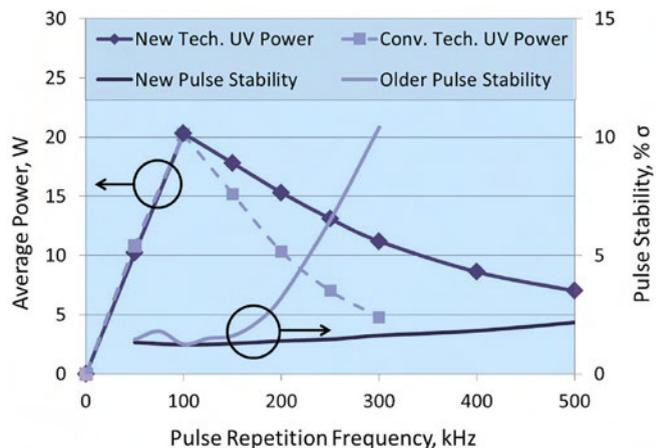
Figure 1: Advanced UV light conversion leads to high power and high-pulse energy stability well beyond the nominal pulse frequency.
