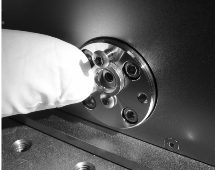
Figure 8-2: Loosen the top retaining screw.
