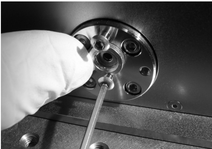
Figure 8-3: Loosen the bottom retaining screw.
