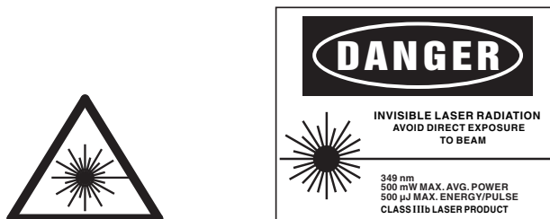
Figure 2-1: These standard safety warning labels are appropriate for use as entry warning signs (EN 60825-1, ANSI Z136.1 Section 4.7).
