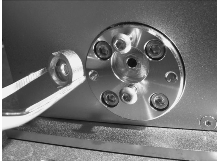
Figure 8-4: Remove the window assembly.
