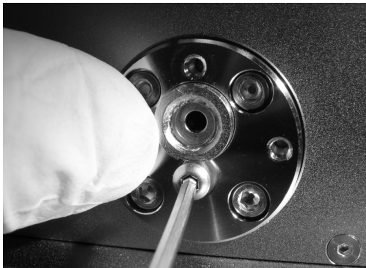
Figure 8-5: Replace the window assembly.
