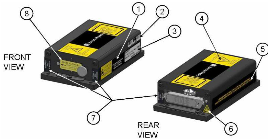
FIGURE 4: Location of Labels on the Laser Head
