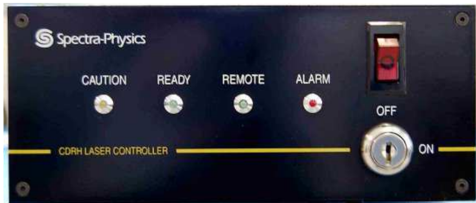
FIGURE 13: Location of status LEDs and switches on the power supply.
