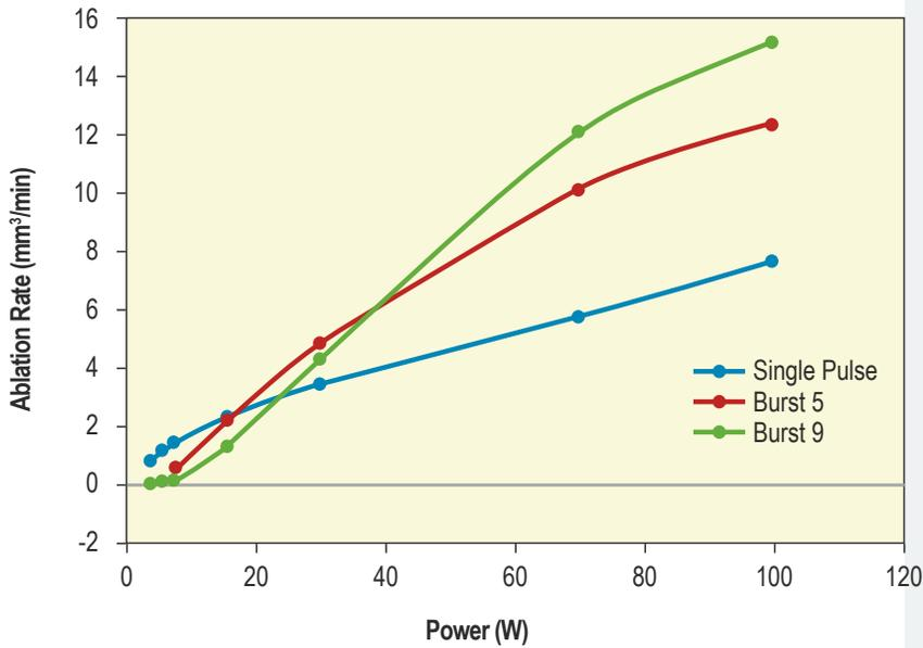
► **Figure 3:** Volumetric ablation rate in polycrystalline diamond (PCD) versus average power for single pulse, five-pulse burst and nine-pulse burst operation. ►
