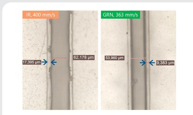
Figure 4: IR vs. green comparison photos of multi-pass cutting in 125  $\mu\text{m}$  thick PET.
