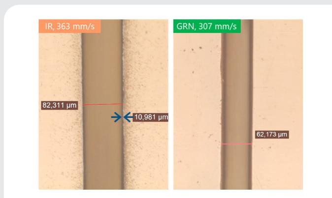
Figure 3: Excellent quality, minimal HAZ for multi-pass cutting of 125  $\mu\text{m}$  thick PI with IR and green wavelengths.
