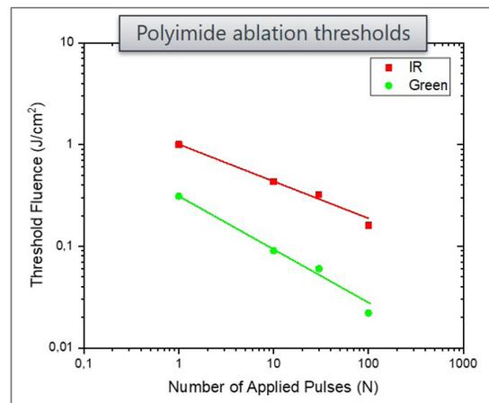
Figure 1: Single- and multi-pulse ablation thresholds in Polyimide.
