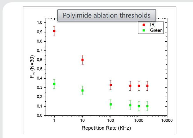
Figure 2: PRF-dependent threshold reduction in polyimide with 30 applied pulses.
