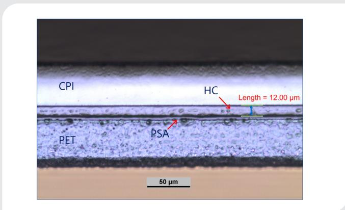
Figure 5. Cross section view of high quality cut in 50  $\mu\text{m}$  clear PI and PET, 12  $\mu\text{m}$  HC, and ~4  $\mu\text{m}$  PSA.
