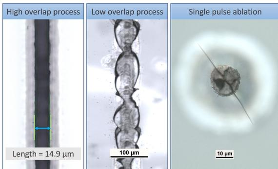
Figure 3. In the  $12 \mu\text{m}$  hard coat film, high-overlap process with closely spaced pulses leads to dramatic quality improvement.
