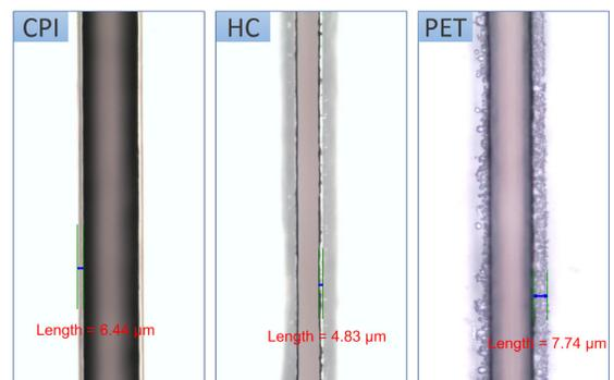
Figure 4. Microscope photos show ps UV laser cuts in clear PI (left), HC (middle), and PET (right) for a layer-specific cutting process with an overall (net) cutting speed of  $>400 \text{ mm/s}$ .
