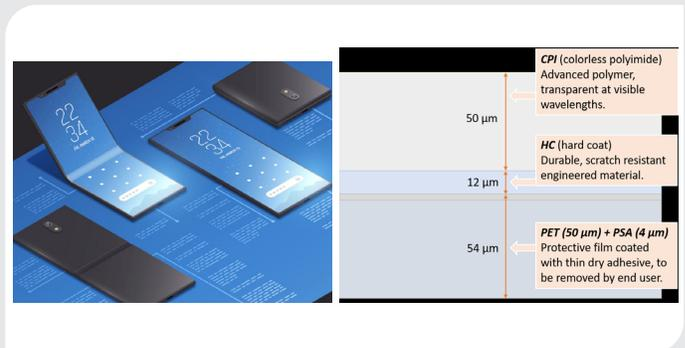
Figure 1. Left – Flexible displays enable foldable phones, a transformative development in mobile device technology. Right – Layer structure diagram of the material stack studied in this applications note.
