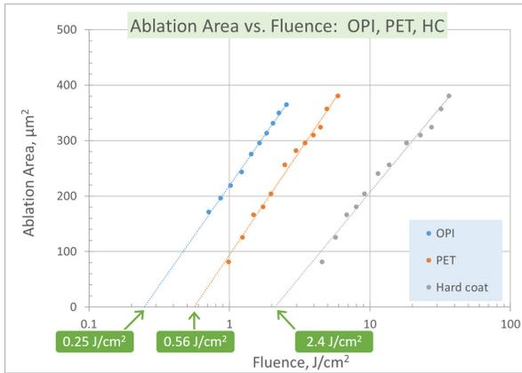
Figure 2. Plot of ablated area vs. laser fluence shows the disparity in thresholds for the three materials in the stack to be cut.
