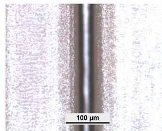
Figure 3. Full cut in 45–50  $\mu\text{m}$  thick bare LCP sheet material with a single pass at 1.0 m/s scan speed.
