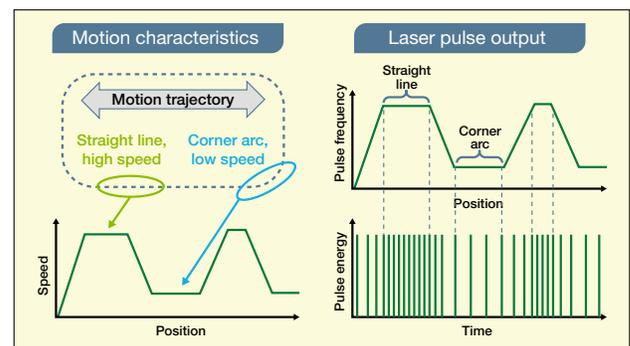
Figure 1. PSO control allows for constant spacing of constant-energy laser pulses on a material throughout a variable-speed trajectory, such as a rounded-corner rectangle.
