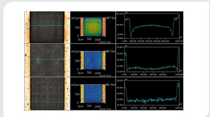
Figure 3. 3D confocal imagery and analysis of stainless steel engraving when using free running (top), skywriting (middle), and PSO (bottom) techniques.
