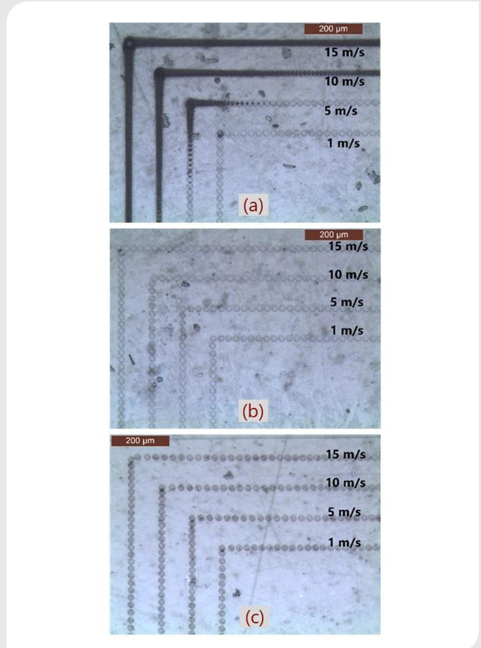
Figure 2. Microscope images showing one corner of a  $1 \times 1$  mm square processed with a UV ultrafast laser with (a) free running, (b) skywriting and (c) PSO techniques.
