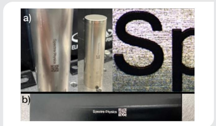
Figure 5. a) black marking on a battery pack and b) white marking of anodized aluminum
