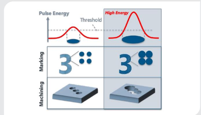
Figure 2. High pulse energies can enable improved visibility of laser markings and increased throughput in micromachining
