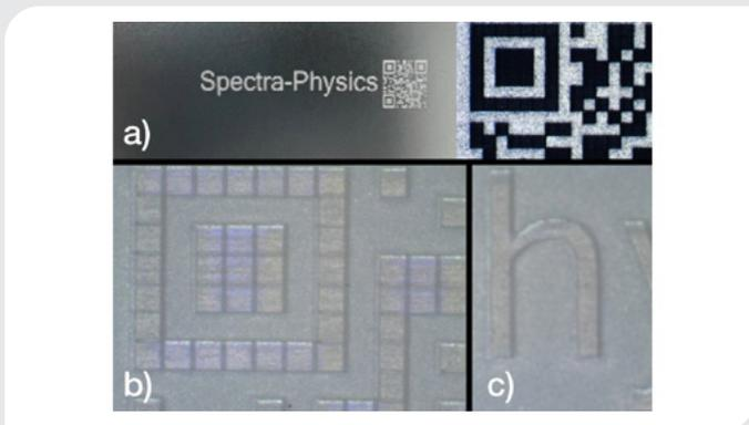
Figure 3. Marking of a) silicon wafers and engraving of b) 2D-matrix codes and c) characters in ceramics
