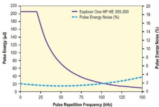
Figure 1. Explorer One HP Energy Curve
