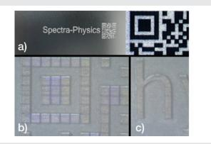
Figure 3. Marking of a) silicon wafers and engraving of b) 2D-matrix codes and c) characters in ceramics
