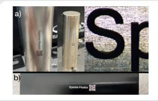
Figure 5. a) black marking on a battery pack and b) white marking of anodized aluminum
