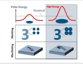
Figure 2. High pulse energies can enable improved visibility of laser markings and increased throughput in micromachining
