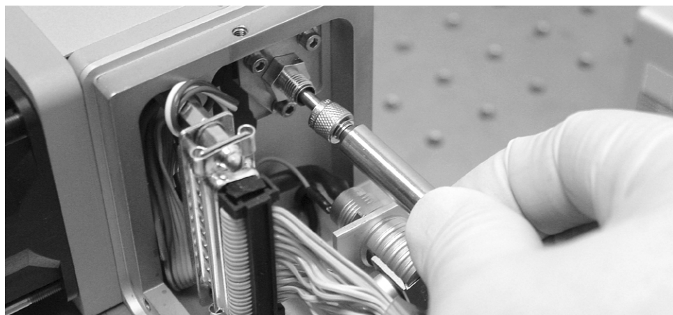
Figure 4-3: Fiber Connection to Laser Head
