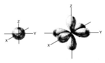
Figure 3-1: Electrons occupy distinct orbitals that are defined by the probability of finding an electron at a given position, the shape of the orbital being determined by the radial and angular dependence of the probability.
