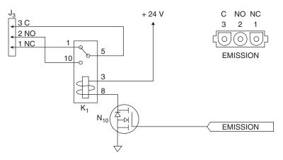
Figure 4-8: The Model J40 or J80 Emission Connector Circuit
