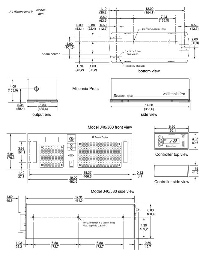
Figure 3-10: Outline Drawings for Laser Head, Controller and Power Supply
