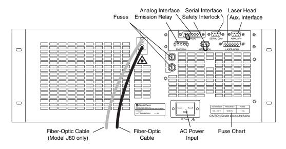
Figure 5-9: The rear panel of the Model J40/J80 power supply
