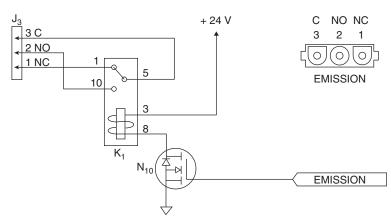
Figure 2-5: The EMISSION Relay Connector Schematic
