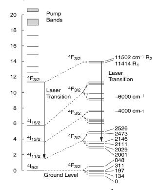
Figure 3-4: Energy Level Scheme for the Nd<sup>3+</sup> Ion
