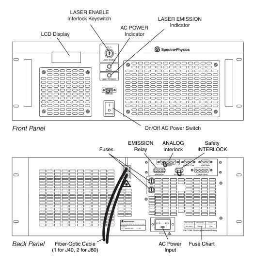
Figure 2-3: Safety devices on the Model J40 or Model J80 power supply
