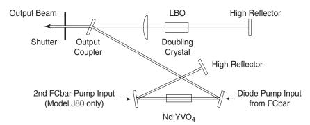
Figure 3-9: Optical Design of the Millennia Pros Laser Head
