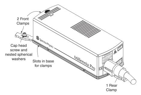
**Figure 5-2: Laser head mounting clamps and base slots**
