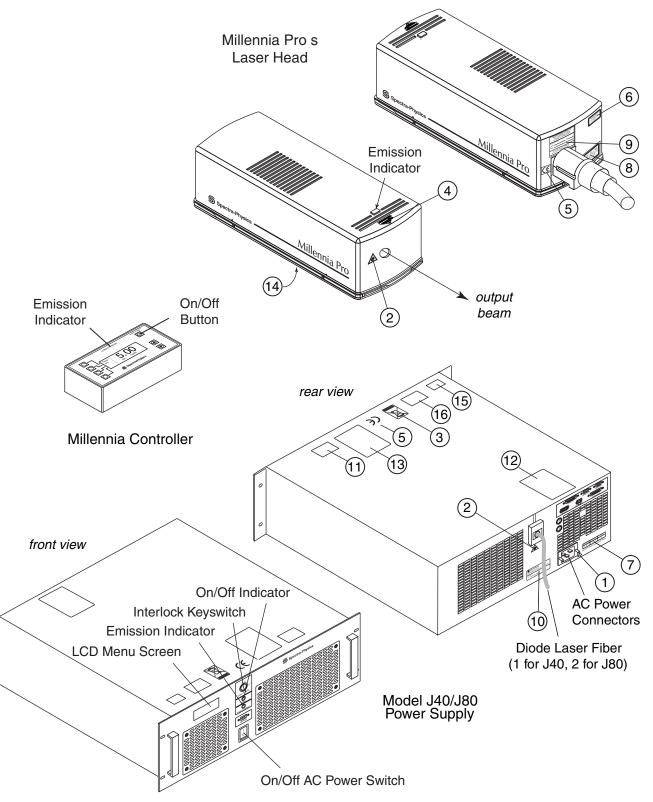
Figure 2-8: CE/CDRH Radiation Control Drawing
