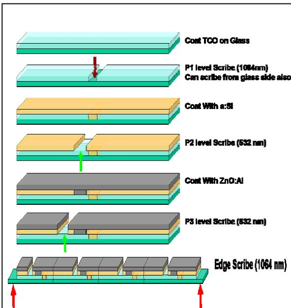
Figure 8. Typical process steps in manufacturing of a-Si based thin film solar cell panel.
