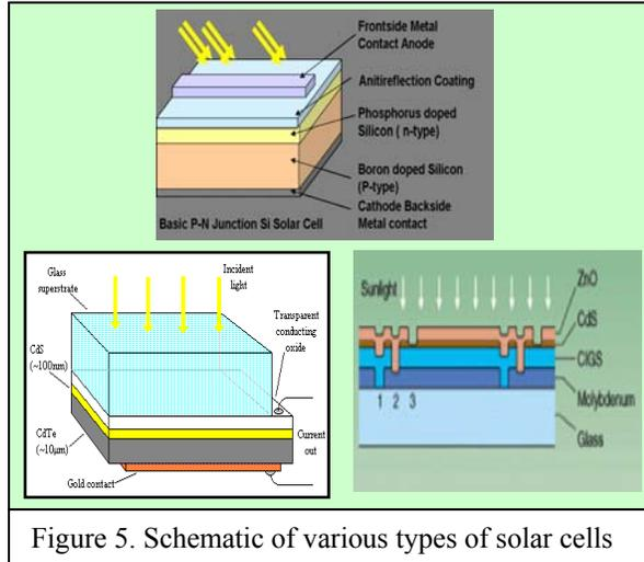
Figure 5. Schematic of various types of solar cells
