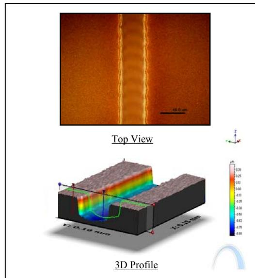
Figure 9. P1 layer ITO scribed using 1064 nm, Hippo<sup>TM</sup> H10-106Q laser at 1.25 m/s.
