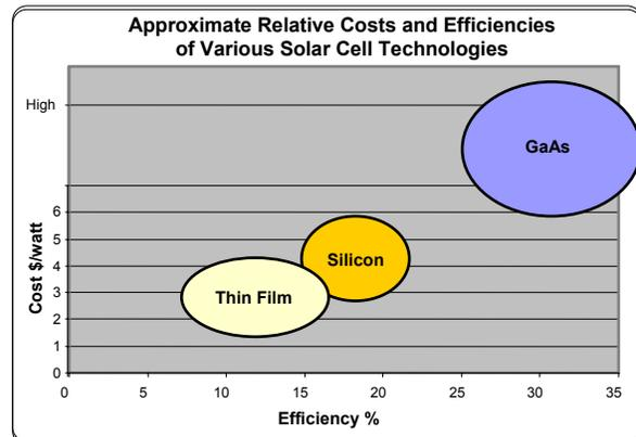
Figure 4. Relative cost and efficiency of various solar cell technologies.
