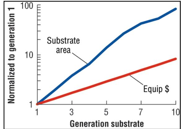
Figure 6. Scaling of FPD substrate area Vs equipment cost.
