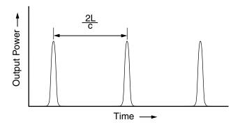
Figure A-1: Typical output of a mode-locked laser, where *L* is the cavity length and *c* is the velocity of light.
