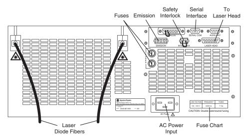
Figure 4-5: The Model J40 Power Supply Rear Panel
