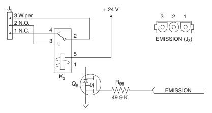
Figure 2-4: The EMISSION Connector Schematic
