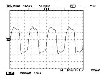
Figure 4-2: Sample waveform supplied by the 40 MHz connector into a  $1 \text{ M}\Omega$  oscilloscope trigger input.
