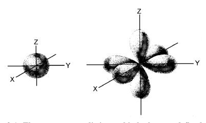
Figure 3-1: Electrons occupy distinct orbitals that are defined as the probability of finding an electron at a given position. The shape of the orbital is determined by the radial and angular dependence of this probability.
