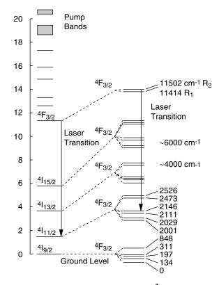
Figure 3-4: Energy Level Scheme for the Nd<sup>3+</sup> Ion.
