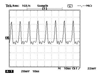
Figure 4-3: Sample waveform from the 80 MHz connector into a 50  $\Omega$  oscilloscope input.
