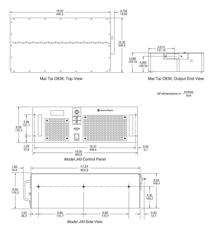
Figure 3-12: Outline Drawing, Mai Tai OEM Laser Head and Model J40 Power Supply
