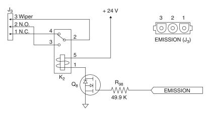
**Figure 5-4: The EMISSION Connector Schematic**
