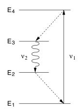
Figure 3-2: A Typical Four-level Transition Scheme
