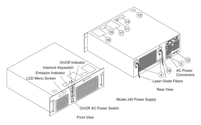
Figure 2-8: CE/CDRH Radiation Control Drawing, *Model J40* Power Supply (labels shown on page 2-10)
