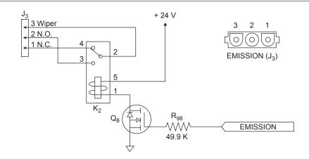
Figure 4-8: Model J40 Emission Connector Circuit
