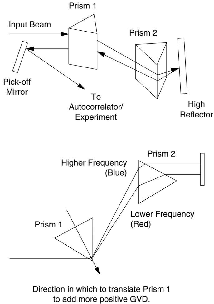
**Figure B-3: Using two prisms to compensate for positive GVD.**
