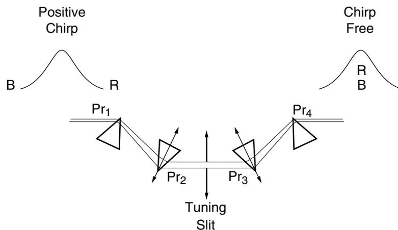
**Figure A-6: A four prism sequence used for dispersion compensation. An input pulse with a positive chirp (red frequencies at the leading edge of the pulse) experiences negative GVD (red frequencies have longer group delay time) in the prism sequence. The net effect is that the prism sequence compensates for the positive GVD and produces a pulse which has no chirp.**
