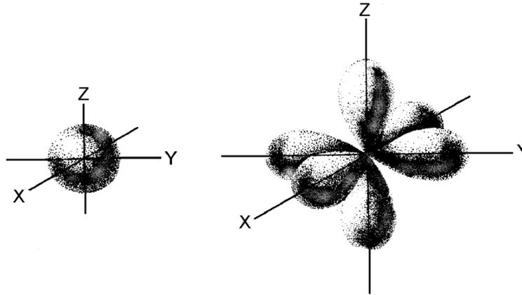
**Figure 3-1: Electrons occupy distinct orbitals that are defined as the probability of finding an electron at a given position. The shape of the orbital is determined by the radial and angular dependence of this probability.**
