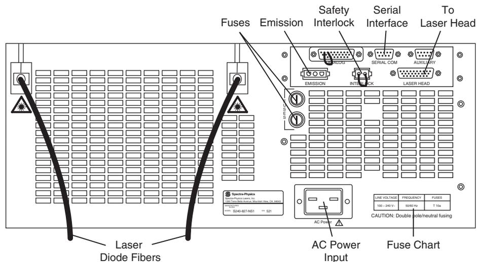
**Figure 4-5: The Model J40 Power Supply Rear Panel**
