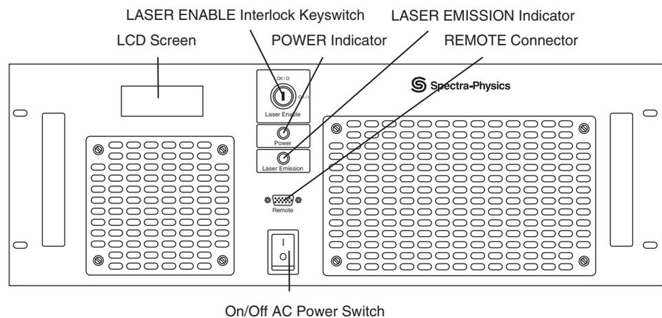
**Figure 4-4: The *Model J40* Power Supply Front Panel**
