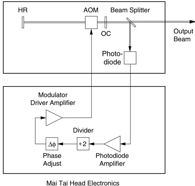
**Figure A-4: Configuration of the electronics for a regenerative mode-locked laser.**
