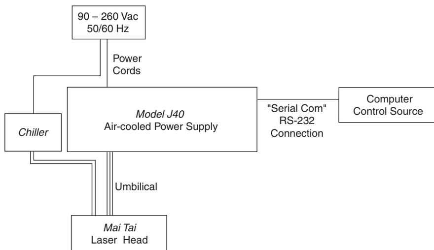
**Figure 5-1: The *Model J40* Interconnect Drawing**
