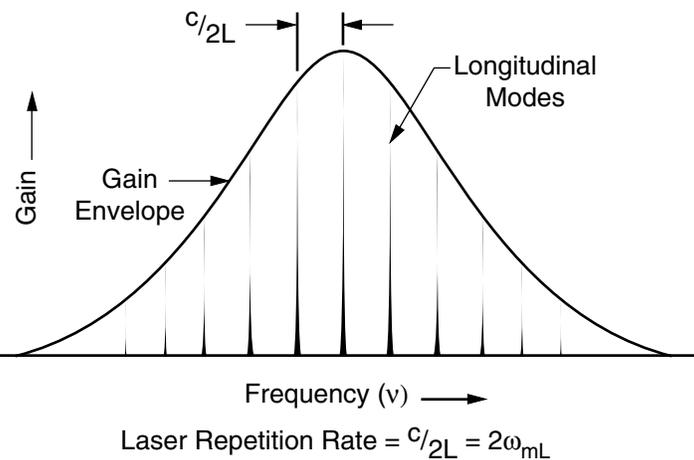
**Figure A-3: Amplitude and frequency of longitudinal modes in a mode-locked laser.**
