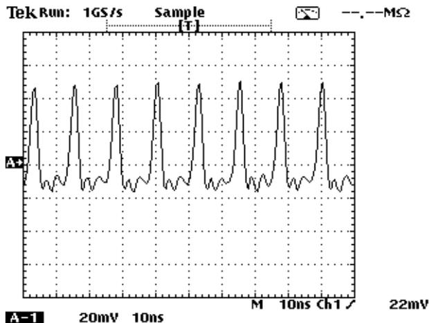
**Figure 4-3: Sample waveform from the 80 MHz connector into a 50  $\Omega$  oscilloscope input.**
