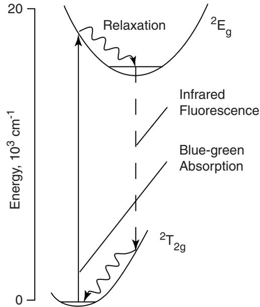
**Figure 3-8: Absorption and emission spectra of Ti:sapphire**
