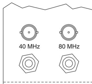
**Figure 4-1: The umbilical attachment panel showing the 40 MHz and 80 MHz BNC connectors.**
