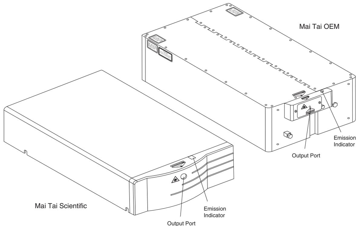
**Figure 2-3: Laser Head Emission Indicator**
