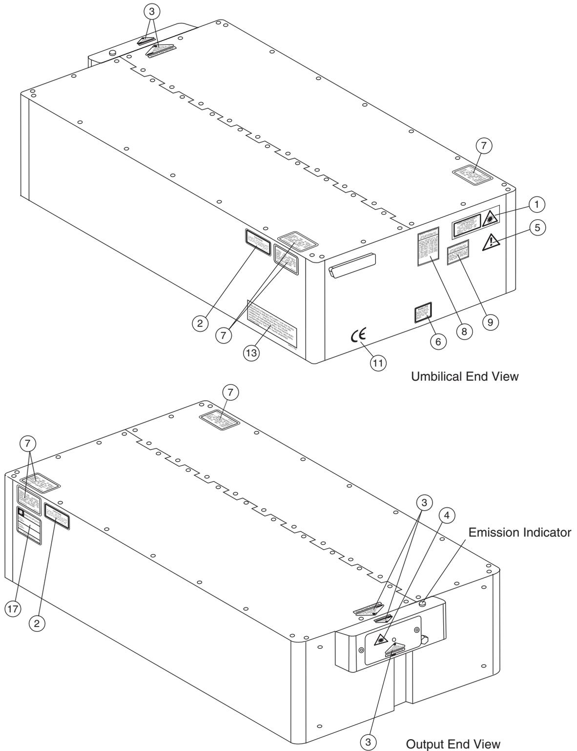
**Figure 2-6: CE/CDRH Radiation Control Drawing, OEM Version (labels shown on page 2-10)**
