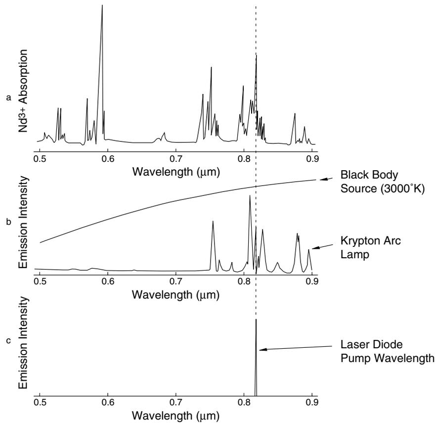
**Figure 3-5: Nd<sup>3+</sup> absorption spectra compared to emission spectra of (a) a Black Body Source, (b) a Krypton Arc Lamp and (c) a Laser Pump Diode.**
