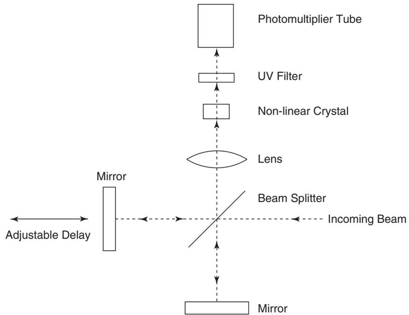
**Figure B-1: Interferometric (Collinear) Autocorrelation**
