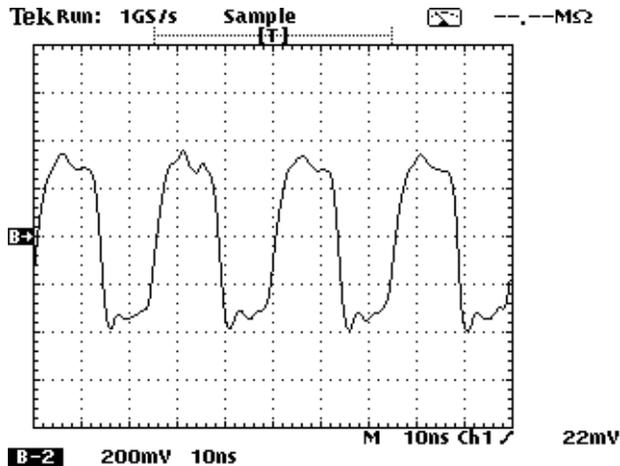
**Figure 4-2: Sample waveform supplied by the 40 MHz connector into a 1 M $\Omega$  oscilloscope trigger input.**
