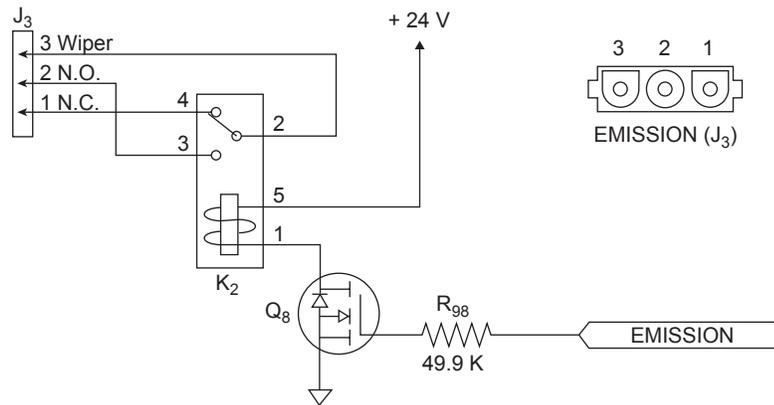
**Figure 4-8: Model J40 Emission Connector Circuit**
