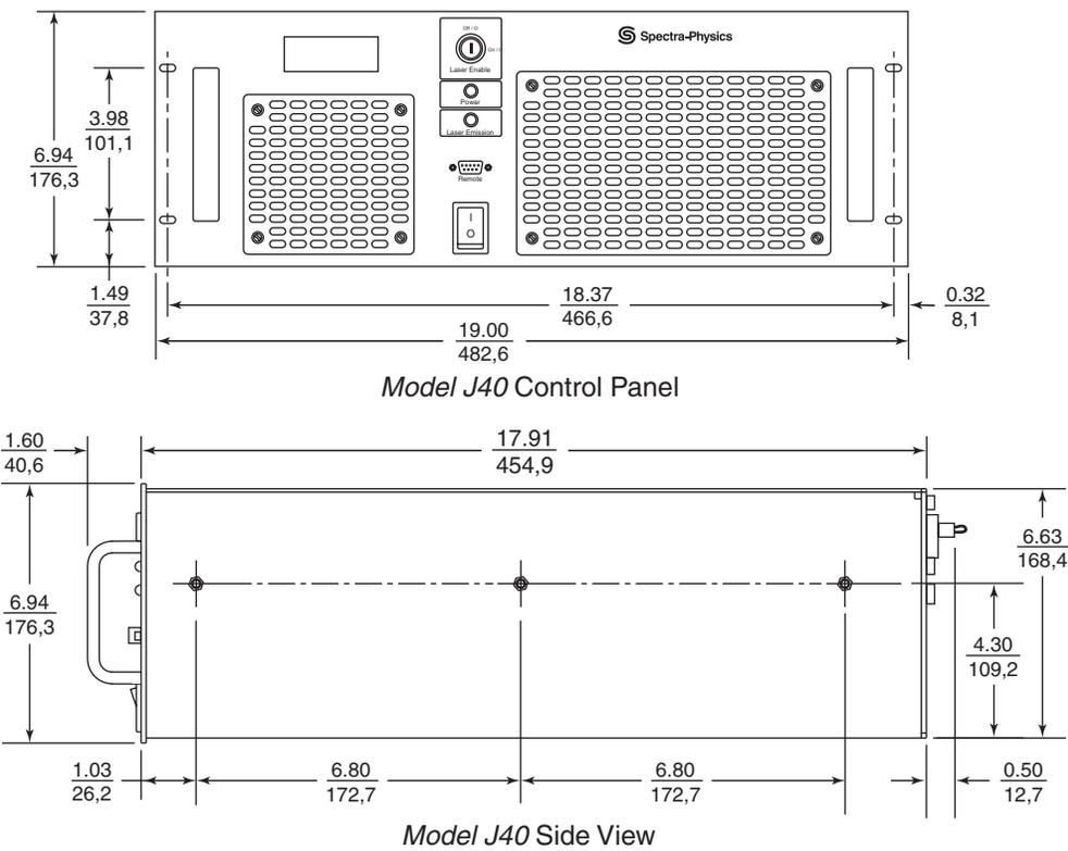
Figure 3-12: Outline Drawing, *Mai Tai* OEM Laser Head and *Model J40* Power Supply
