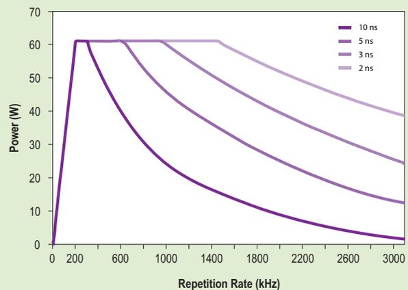
1. Quasar UV60 specified power is >60 W at 300 kHz 10 ns. Quasar UV60-Turbo specified power is >38 W at 3 MHz 2 ns. Other points on graph are not a guaranteed or warranted specification.
