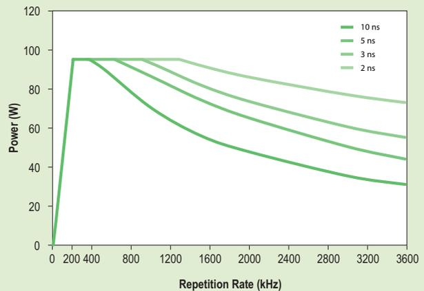
1. Quasar GR95 specified power is >95 W at 200 kHz 10 ns. Quasar GR75 specified power is >75 W at 200 kHz 10 ns. Other points on graph are not a guaranteed or warranted specification.
