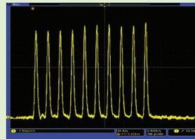
10 x 5 ns sub-pulses (Burst Mode)<sup>1,2</sup>
