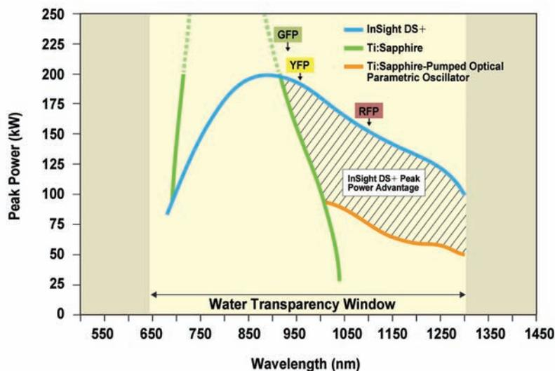
**Figure 1.** Legacy Ti:sapphire platforms and their optical parametric oscillator extensions deliver limited power above 900 nm, where most of today’s multiphoton excited fluorescence imaging takes place. New platforms such as InSight DS+ are optimized for high peak power above 900 nm to drive much increased fluorescence and deeper penetration, as is illustrated by the shaded area. Courtesy of Spectra-Physics.
