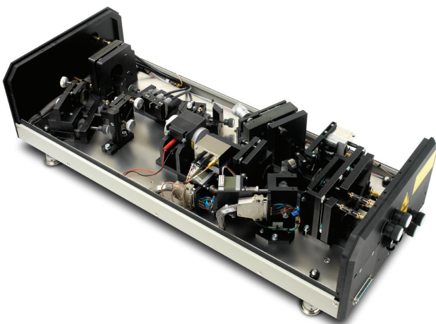
Open cavity Matisse 2 TX showing intra-cavity EOM for fast cavity length stabilization
