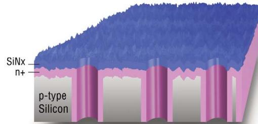
Step 2: The wafer goes through a gas phase diffusion step to create the n+ emitter. The via holes function to "wrap" the emitter through (EWT) to the rear surface so that both the front side grid and front-to-back interconnections can be eliminated.
