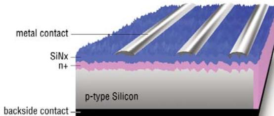
Step 5: This step shows the addition of screen printed metal paste that, once fired, forms the busbars and finger gridlines of the front surface contacts.
