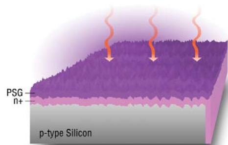
Step 2: Thermal diffusion of phosphorus doping – wafers are heated in a furnace with  $POCl_3$  gas to create the n+ emitter via diffusion.
