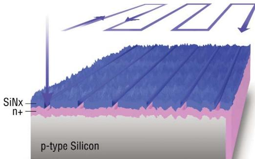
Step 1: After deposition of the ARC layer, the laser is scanned over the front surface and selectively ablates the ARC layer in the pattern of the front side grid.
