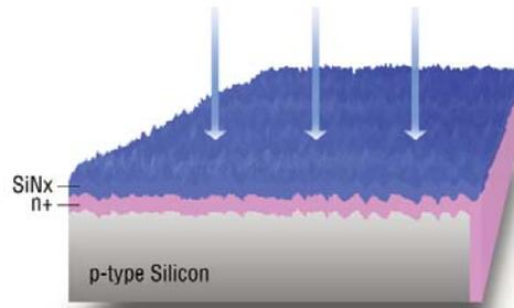
Step 4: PECVD of an anti-reflection (AR) thin film dielectric coating of Silicon Nitride ( $SiNx$ ) or alternatively oxidation to form a  $SiO_2$  AR layer on the front surface to further improve light absorption.
