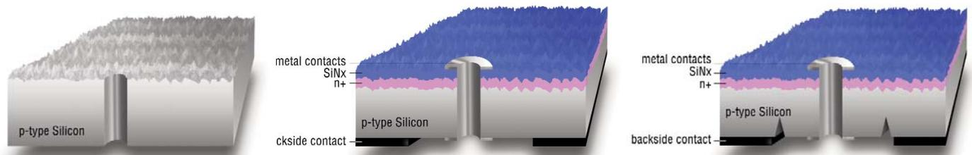
*Step 1: Via holes are drilled through the silicon wafer prior to thermal diffusion of the phosphorus doping.*
