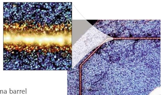
Crystalline silicon solar cell edge isolation (with close up view) using a Pulseco 355 nm DPSS Q-switched laser. 20  $\mu\text{m}$  scribe width and 10  $\mu\text{m}$  scribe depth.
