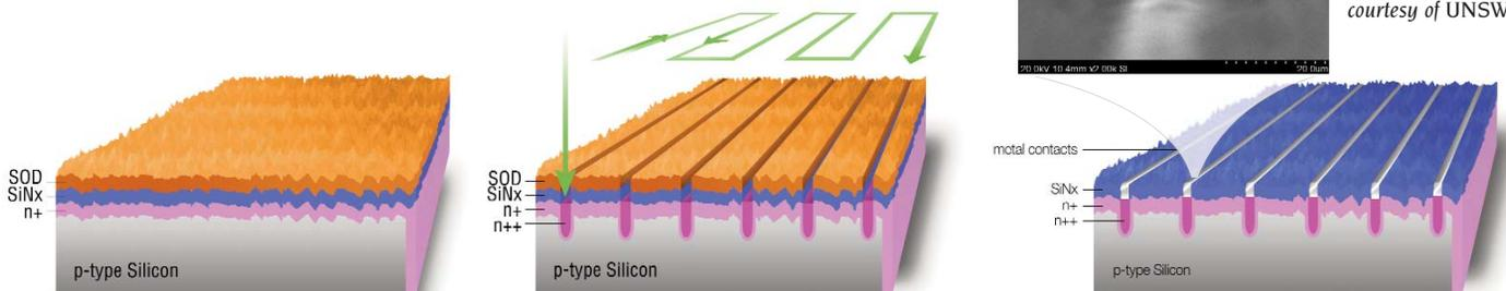
Step 1: After ARC deposition, a thin phosphorous coating is applied to the wafer front side.
