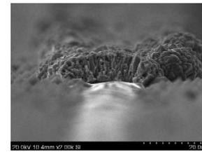
SEM image of copper-plated LDSE finger line. Image courtesy of UNSW.
