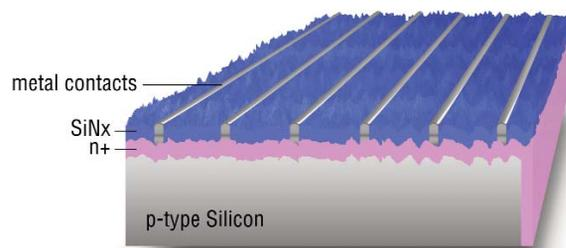
Step 2: The cells are screen printed and furnace fired to complete the fingers and busbars, which bond directly with the n+ layer for better electrical contact.
