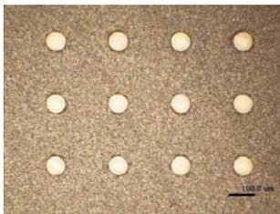
*200 μm thick c-Si wafer drilled with 50-60 μm diameter.*
