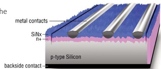
After the screen printing and furnace firing steps, cell edges are laser scribed to electrically isolate the back of the cell from the front.
