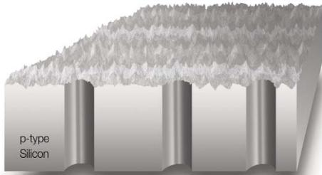
Step 1: Via holes are drilled through the silicon wafer prior to thermal diffusion of the phosphorus doping.
