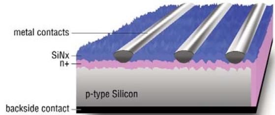
Step 6: Heating or “firing” of screen printed metal paste gridlines results in the lines melting through the thin insulating layer of  $SiNx$ , to effectively make electrical contact with the underlying silicon layer, in this case the n+ emitter.
