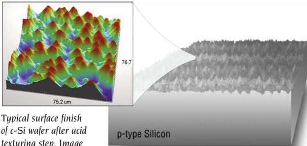
Typical surface finish of c-Si wafer after acid texturing step. Image courtesy of Veeco Instruments.
