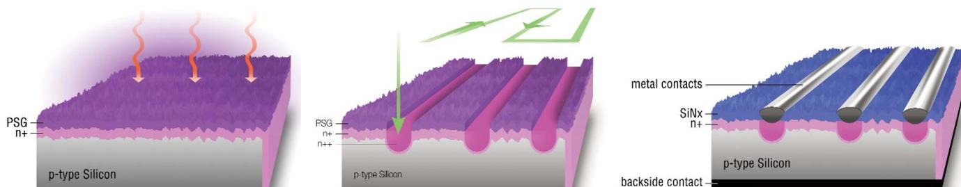
Step 1: During the thermal diffusion process, a layer of phosphor silicate glass (PSG) is formed.
