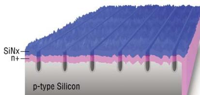
Step 1: After the deposition of the ARC layer, a deep groove is laser scribed into the silicon.
