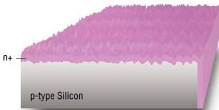
Step 3: The hydrofluoric (HF) acid etch process removes the unwanted layer of phosphor silicate glass (PSG) produced during the diffusion step.
