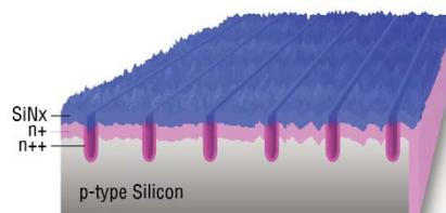
Step 2: After scribing, the walls of these grooves are heavily doped, forming n++ type groove walls.
