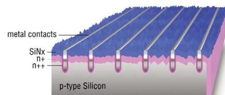
Step 3: The grooves are filled with plated metal contacts (vertical busbars) then screen printed (fingers) and furnace fired to complete the front side grid.
