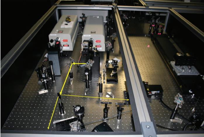
Figure 4. Output beam of TOPAS is picked off and sent to photodiode.
