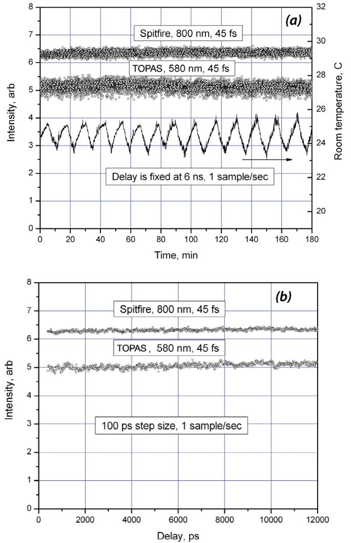
Figure 5. (a) The output of the slave amplifier and TOPAS at fixed delay. (b) Stability of the output of slave amplifier and TOPAS vs. delay.
