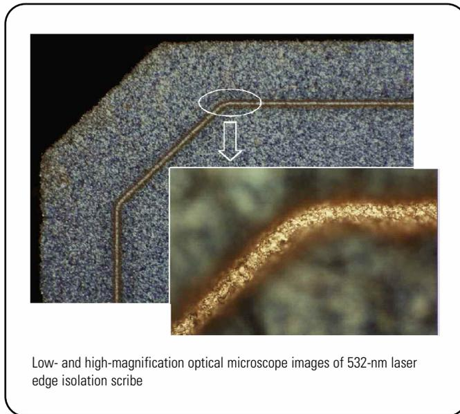
Low- and high-magnification optical microscope images of 532-nm laser edge isolation scribe
