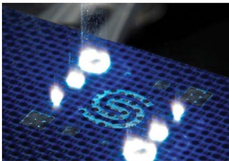
Figure 1: Lasers are increasingly finding use for cutting, drilling, and texturing CFRP components.
