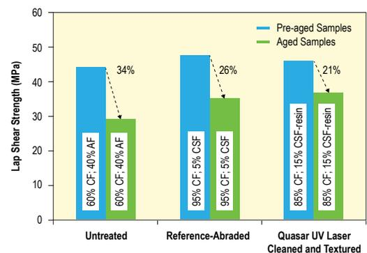
CF = Cohesive Failure, AF = Adhesive Failure, CSF = Cohesive Substrate Failure
