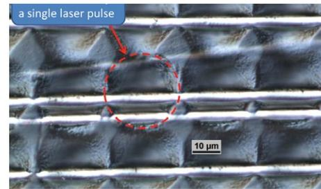
Figure 3: Laser treated surface of CFRP shows clean texturing of the polymer matrix without damage to the individual carbon fibers.
