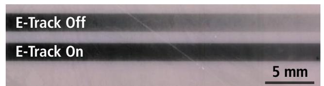
Figure 4: E-Track can compensate effects due to uneven surfaces
