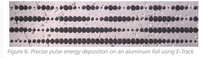
Figure 6: Precise pulse energy deposition on an aluminum foil using E-Track
