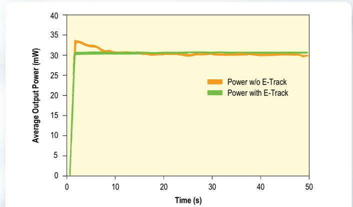
Figure 2: Overshoot compensation controlled by E-Track while gating the laser
