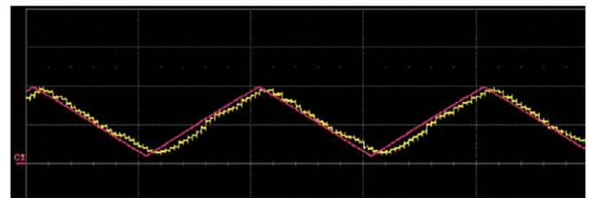
Figure 3: Modulated pulse energy levels controlled by E-Track monitored on an oscilloscope
