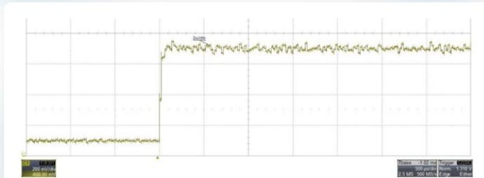
Figure 1: Pulse energy change controlled by E-Track, monitored on an oscilloscope. Each single step of the signal represents the energy of one pulse
