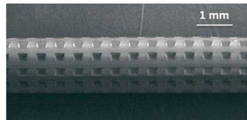
Figure 3: SEM (scanning electron micrograph) image showing a detailed view of a modified area. Shown are machined defects with a footprint of  $250 \times 250\ \mu\text{m}$  and a depth of  $65\ \mu\text{m}$ . The bottom surface is in the fiber core so that light is decoupled because the total internal reflection is prevented.
