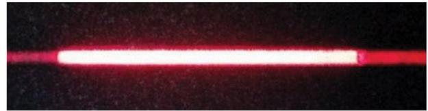
Figure 5: Photograph of an optical fiber diffuser with a length of 55.5 mm fabricated with the Spirit femtosecond laser. Light is decoupled out of the optical fiber at the modified areas and results in a uniformly diffused illumination.
