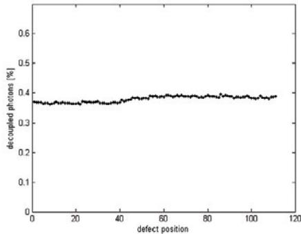
Figure 4: Decoupled photons per defect at the linearized diffusor. Number of defects  $N=111$ , footprint =  $250 \times 250 \mu\text{m}$ , pitch =  $500 \mu\text{m}$ .
