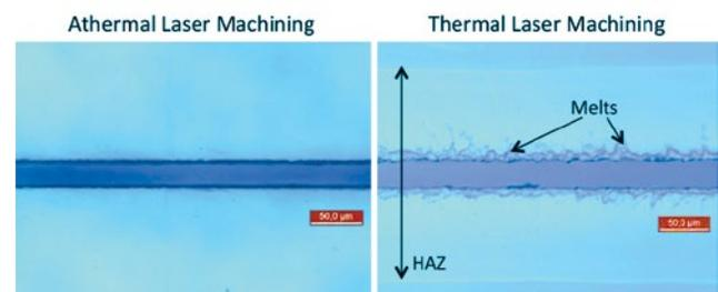
Figure 2. Microscope images of typical cutting kerfs in PLLA obtained in athermal (left) and thermal (right) laser machining regimes.
