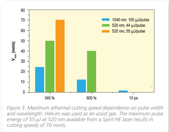
Figure 3. Maximum athermal cutting speed dependence on pulse width and wavelength. Helium was used as an assist gas. The maximum pulse energy of 55 µJ at 520 nm available from a Spirit HE laser results in cutting speeds of 70 mm/s.
