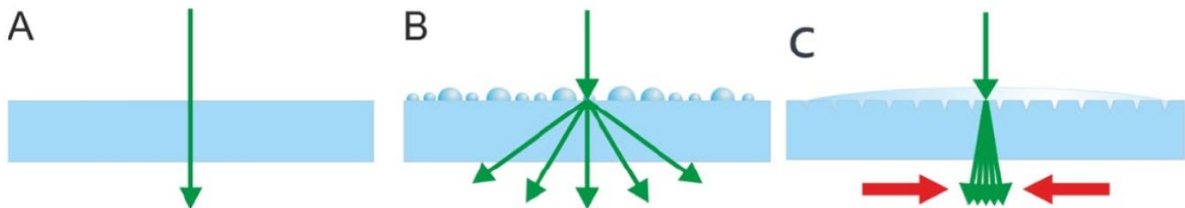
Figure 1. Light scattering on dry (A) and fogged (B) glass surfaces. Anti-fogging surfaces have super-hydrophilic property to provoke spreading of the fog droplets on the surface (C). As a consequence, light scattering reduces in the wetted state (indicated by the red arrows).
