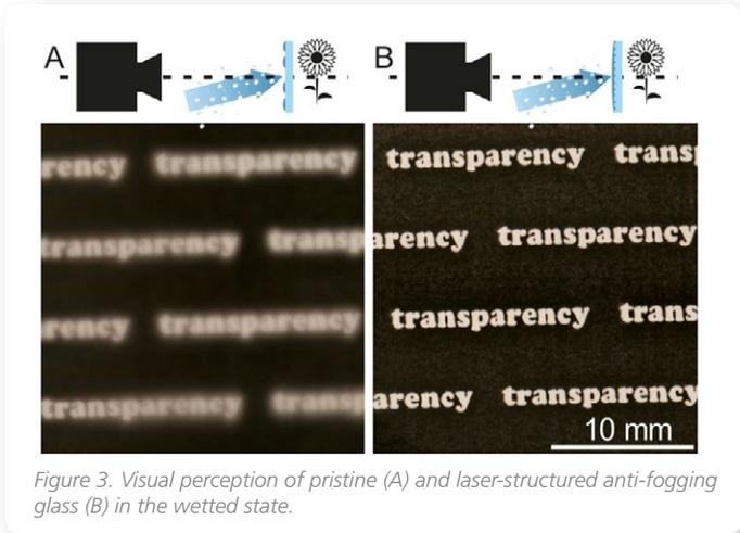
Figure 3. Visual perception of pristine (A) and laser-structured anti-fogging glass (B) in the wetted state.
