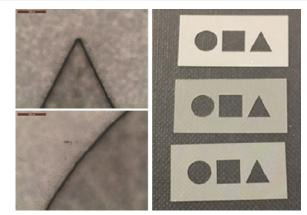
Figure 4. Microscope images of PET plastic ribbon cut using femtosecond Spirit 1030-100-SHG laser at 515 nm. An average power of 50 W at 515 nm allows cutting of 75 µm thick film with a cutting speed above 0.4 m/s with superior quality (HAZ < 10  $\mu$ m).
