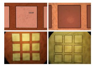
Figure 3. Microscope images of Polyimide (left) and PET (right) plastics cut using Spirit 1030-100-SHG laser from Spectra-Physics. Application of a femtosecond laser with the average power of 100 W at 1030 nm results in a cutting speed above 1 m/s for 75  $\mu$ m thick plastics and very high quality (HAZ < 50  $\mu$ m).
