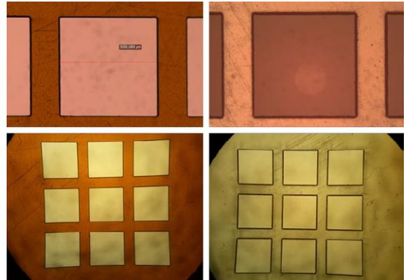
Figure 2. Microscope images of Polyimide (left) and Polyethylene Terephthalate (right) plastics cut using Spirit 1030-100-SHG laser from Spectra-Physics. Application of a femtosecond laser with average power of 100 W at 1030 nm results in cutting speed above 1 m/s for 75  $\mu$ m thick plastics and very high quality (HAZ  $<50$   $\mu$ m).
