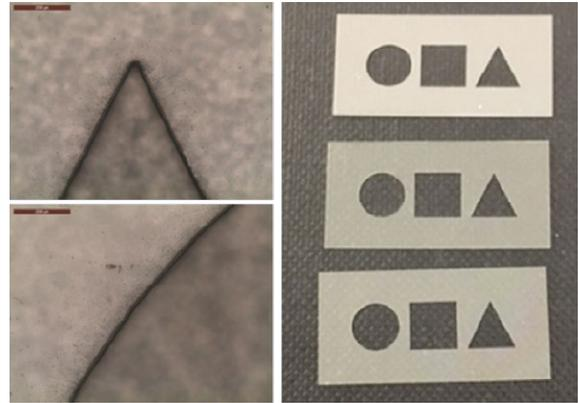
Figure 3. Microscope images of Polyethylene Terephthalate (PET) plastic ribbon cut using a femtosecond Spirit 1030-100-SHG laser at 515 nm. The average power of 50 W at 515 nm results in cutting speeds over 0.4 m/s for 75  $\mu$ m thick PET with superior quality (HAZ <10  $\mu$ m).
