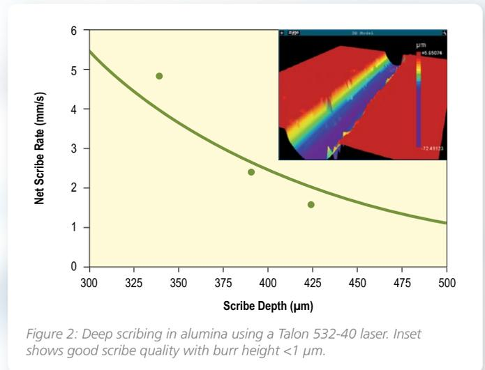
Figure 2: Deep scribing in alumina using a Talon 532-40 laser. Inset shows good scribe quality with burr height <1 µm.
