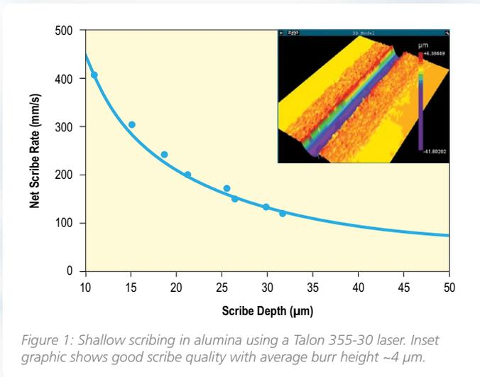
Figure 1: Shallow scribing in alumina using a Talon 355-30 laser. Inset graphic shows good scribe quality with average burr height ~4 µm.
