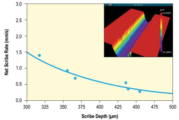
Figure 4: Deep scribing in aluminum nitride using a Talon 355-30 laser. Inset shows excellent scribe quality with negligible burr.
