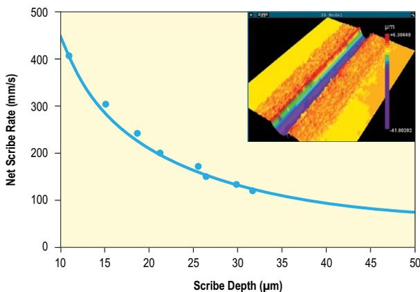
Figure 1: Shallow scribing in alumina using a Talon 355-30 laser. Inset graphic shows good scribe quality with average burr height ~4 µm.
