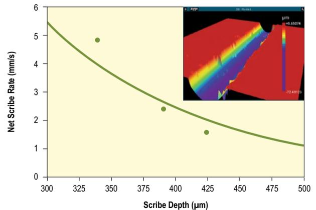
Figure 2: Deep scribing in alumina using a Talon 532-40 laser. Inset shows good scribe quality with burr height <1 µm.
