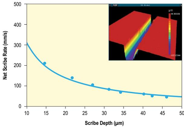
Figure 3: Shallow scribing in aluminum nitride using a Talon 355-30 laser. Inset shows excellent scribe quality with negligible burr.
