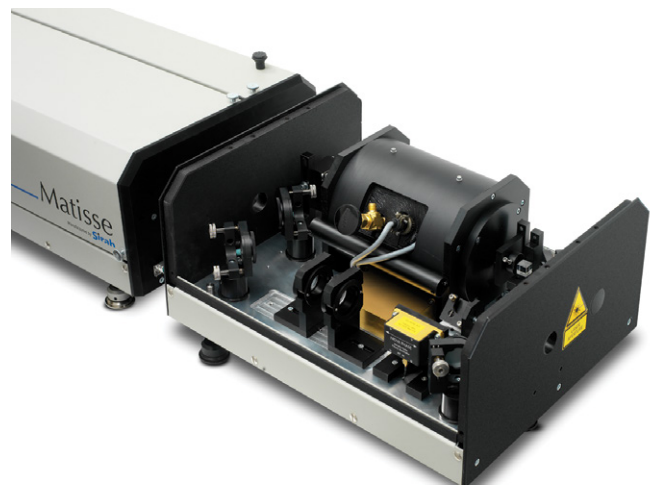
Matisse 2 TX with separate, optional reference cavity with Pound-Drever-Hall feedback scheme
