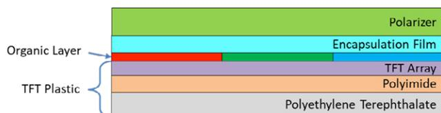
Figure 1. Schematic representation of a flexible OLED structure
