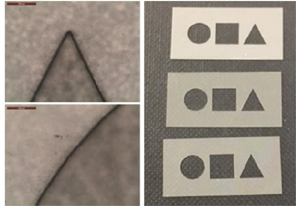
Figure 4. Microscope images of PET plastic ribbon cut using femtosecond Spirit 1030-100-SHG laser at 515 nm. An average power of 50 W at 515 nm allows cutting of 75  $\mu\text{m}$  thick film with a cutting speed above 0.4 m/s with superior quality (HAZ < 10  $\mu\text{m}$ ).
