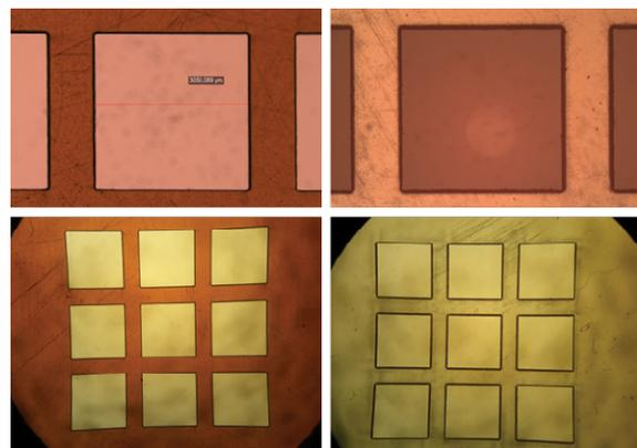
Figure 3. Microscope images of Polyimide (left) and PET (right) plastics cut using Spirit 1030-100-SHG laser from Spectra-Physics. Application of a femtosecond laser with the average power of 100 W at 1030 nm results in a cutting speed above 1 m/s for 75 µm thick plastics and very high quality (HAZ < 50 µm).
