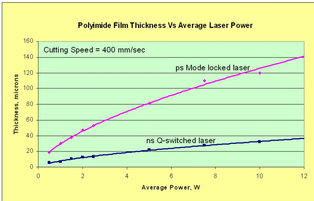
Fig. 7: Comparison of nanosecond and picosecond cutting of polyimide with laser
