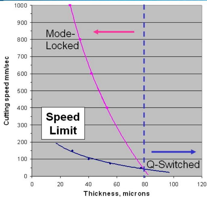
Fig. 2: Polyimide machining comparing scribe depth achieved at a given cutting speed
