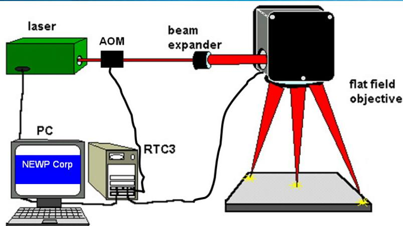
Fig. 1: Experiment Set-up of the scanning beam projection system
