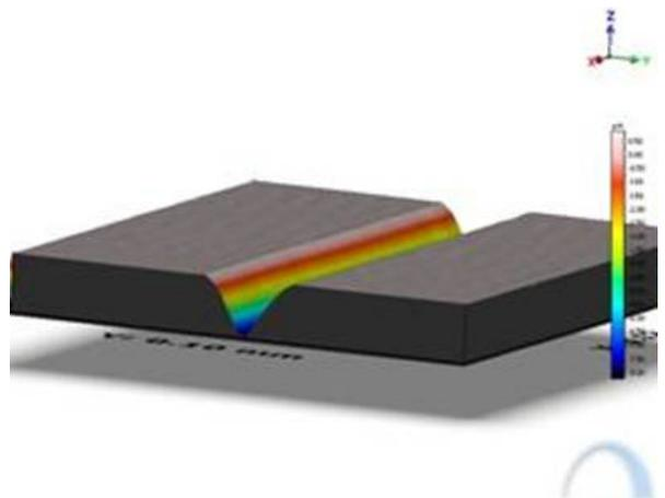
Fig. 5: 9  $\mu$ m deep and 25  $\mu$ m wide groove machined in polyimide
