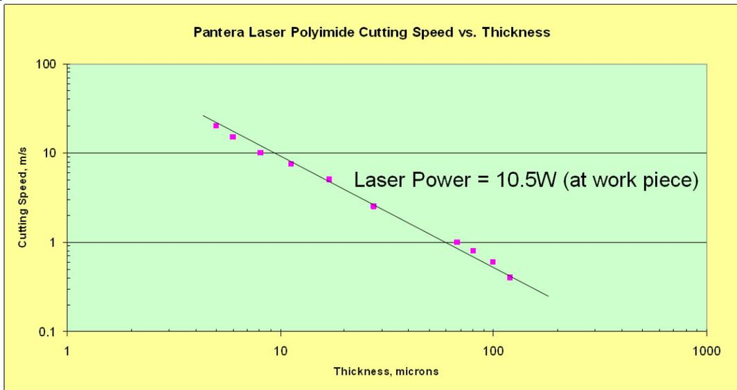
Fig. 6: Cutting speed vs. thickness in Polyimide using a Pantera™ laser
