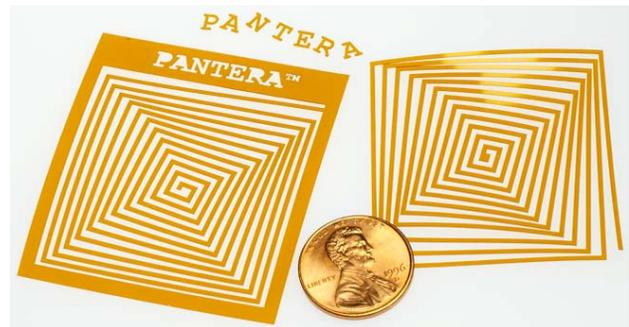
Fig. 4: Polyimide cutting 75 $\mu$ m with 1m/s
