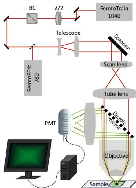
Fig. 1: 2PM with two fixed-WL lasers.  $\lambda/2$  = Lambda-half plate, BC = polarising beam splitter cube, PMT = photo multiplier tube.
