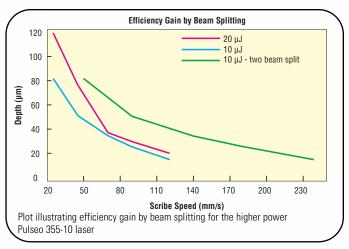
With higher power Pulseo® 355-10 laser system we have shown that the potential gain of up to 75% in processing speed by beam splitting is possible. For 25 µm-deep scribes, a scribing speed of up to 188 mm/sec can be achieved.
