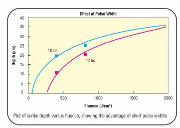
Today's laser products offer ever increasing power levels – and this also holds true for short pulse width, 355 nm wavelength lasers. With this trend, it can be challenging to increasingly utilize this higher power and pulse energy as efficiently as possible. In Spectra-Physics' Industrial Applications Lab, we have explored techniques to increase process efficiency while maintaining quality of Sapphire scribes using different lasers and beam delivery systems.
