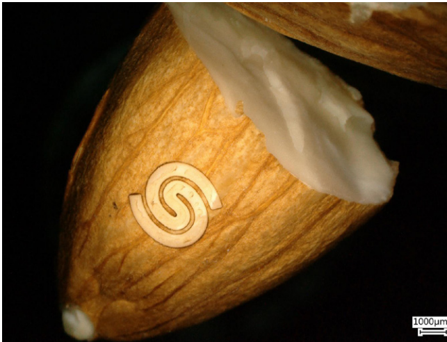
Figure 6 Direct food marking using the Explorer One HP 355-4. The Spectra-Physics logo was marked by ablating the almond shell.
