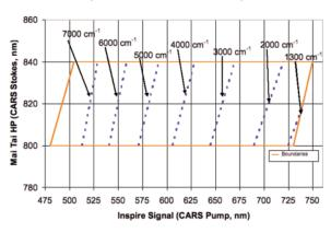
Figure 3: Simultaneous Outputs from the Mai Tai HP and the Inspire OPO Signal. The area within the orange parallelogram indicates wavelength choices that are available for simultaneous output.
