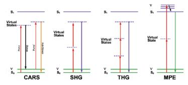
Figure 1: Energy Level Diagrams of Imaging Techniques. Coherent Anti-Stokes Raman Scattering (CARS), Second Harmonic Generation (SHG), Third Harmonic Generation (THG), and Multiphoton Excited Fluorescence (MPEF, here: twophoton excited fluorescence).
