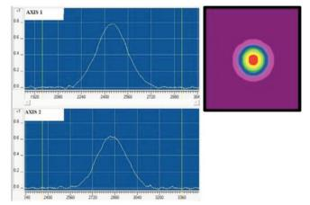
Figure 6: Inspire OPO Idler beam profile at 1,030nm
