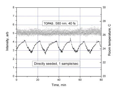
Figure 6. The output stability of TOPAS when pumped by the master amplifier.
