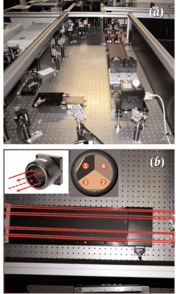
Figure 3. (a) Elevated end view of the delay line. (b) An 8-pass delay line using two retroreflectors. Inset of (b) shows the beam path. The solid line indicates the first and the second passes while the dashed line shows the third and the fourth passes. This pattern is repeated on the second retroreflector adjacent to the first. Also shown is the front view of the retroreflector. The beam path within the retroreflector is not shown.
