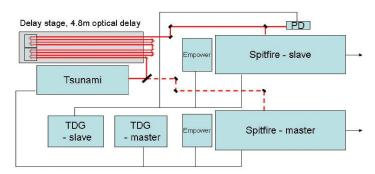
Fig. 1. Block diagram setup for synchronizing two amplifiers with a single oscillator. PD - photodiode; TDG - time delay generator.
