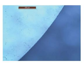
Example of 6.4 mm diameter round camera lens cover window cut from a 0.43 mm thick sapphire wafer with ClearShape process using Spirit laser. The cutting time of <0.5 sec/window can be achieved.
