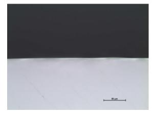
TOP VIEW Top view of the cut edge shows a clean cut quality with minimal chipping (<10  $\mu$ m).
