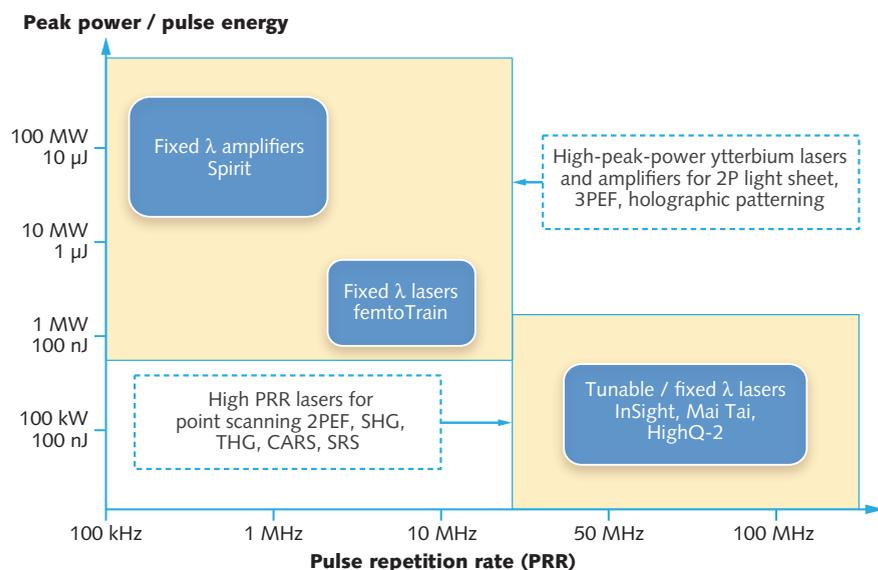
**FIGURE 1.** There is a tradeoff between high repetition rate lasers suitable for point-scanning microscopy, and high peak power lasers suitable for emerging imaging techniques.
