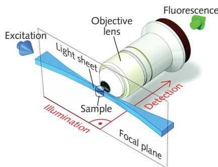
Fluorescence light sheet microscopy uses orthogonal paths for illumination and detection. (Reproduced from Jan Huiskens and Didier Stainier<sup>4</sup>)
