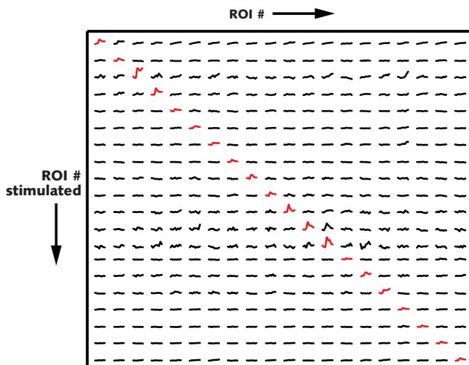
**FIGURE 6.** Spatial selectivity of photostimulation: Calcium signals are only detected for photoactivated neurons (highlighted in red). (Courtesy of Dr. Alan Mardinly, University of California, Berkeley)
