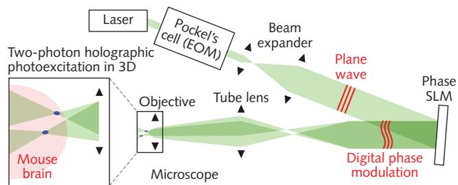
**FIGURE 3.** A two-photon holographic patterning arm, with a spatial light modulator, creates arbitrary 3D photoexcitation in live mouse brain. (Courtesy of Dr. Nicholas Pegard, University of California, Berkeley)
