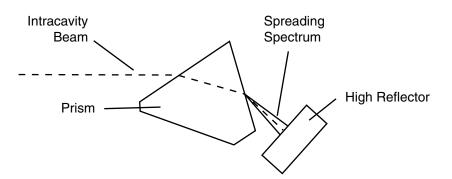
Figure 6-2: Only one line of the cavity beam spread by the prism is at the proper angle to return along the beam path and become amplified.
