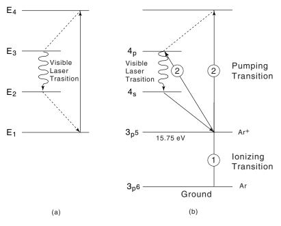
Figure 3-2: A typical four-level laser transition scheme (a) compared to that of visible argon (b). One electron collision ionizes neutral argon, and a second pumps the ion to an excited state.
