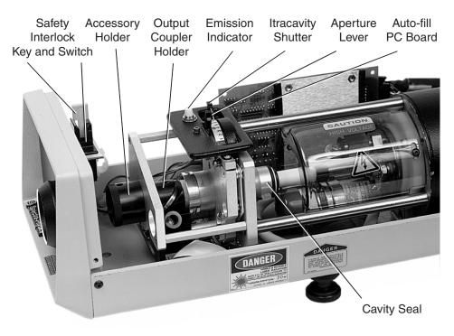
Figure 4-1: Laser Head Interior—Output End
