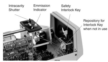
Figure 2-3: Laser Head Safety Interlock Key, Intracavity Shutter, and Emission Indicator
