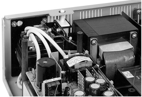
Safety Interlock Switch (shown pulled up in defeat position)
