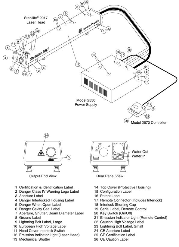
Figure 2-8: CE/CDRH Radiation Control Drawing (refer to the warning labels on next page)
