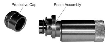
Figure 4-3: The Stabilite 2017 Prism Assembly
