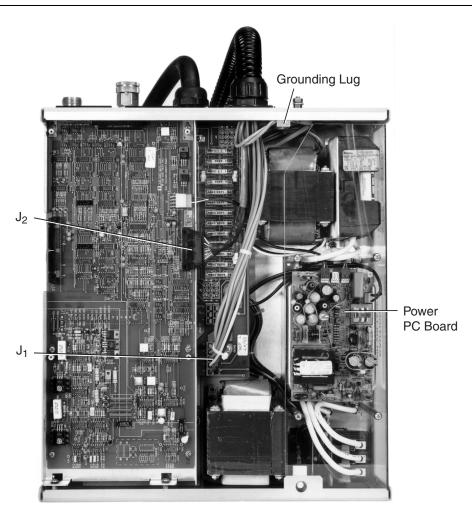
Figure 5-1: Model 2550 Power Supply with the Cover Removed
