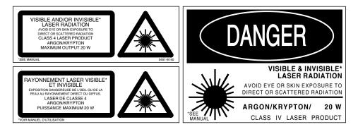
Figure 2-1: These CE and CDRH standard safety warning labels would be appropriate for use as entry warning signs (EN 60825-1, ANSI 4.3.10.1).
