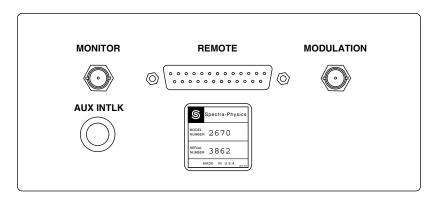
Figure 4-6: Model 2670 Controller Rear Panel
