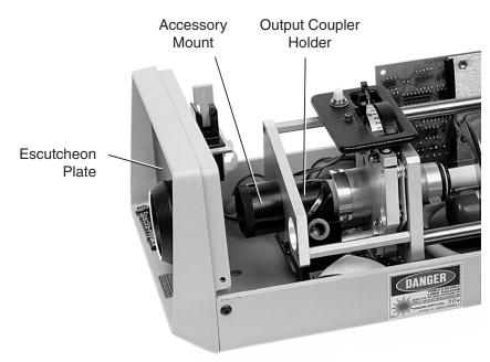
Figure 6-1: The laser head showing the output coupler holder.
