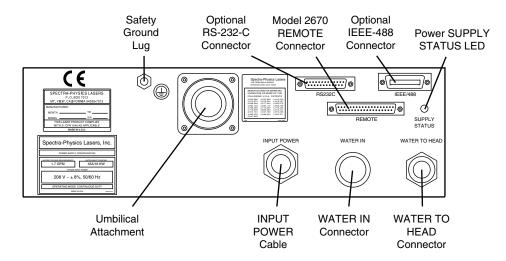
Figure 4-4: Front Panel of the Model 2550 Power Supply
