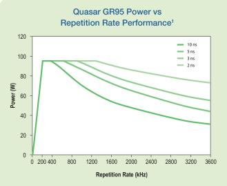
1. Quasar GR95 specified power is >95 W at 200 kHz 10 ns. Quasar GR75 speficifed power is >75 W at 200 kHz 10 ns. Other points on graph are not a guaranteed or warranted specification.
