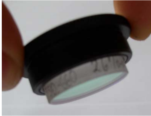
Figure 74: Matisse mirror, squeezed in a metal ring. The mirror will not fall, even when the ring is turned upside down.
