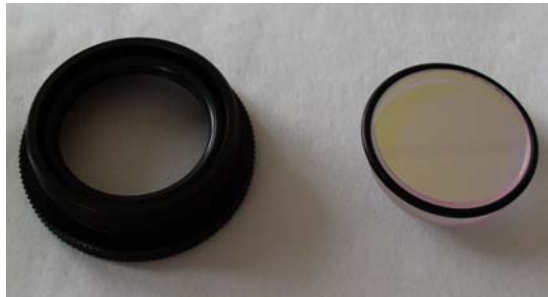
Figure 75: Matisse mirror and mirror mount ring with the two o-rings in place.
