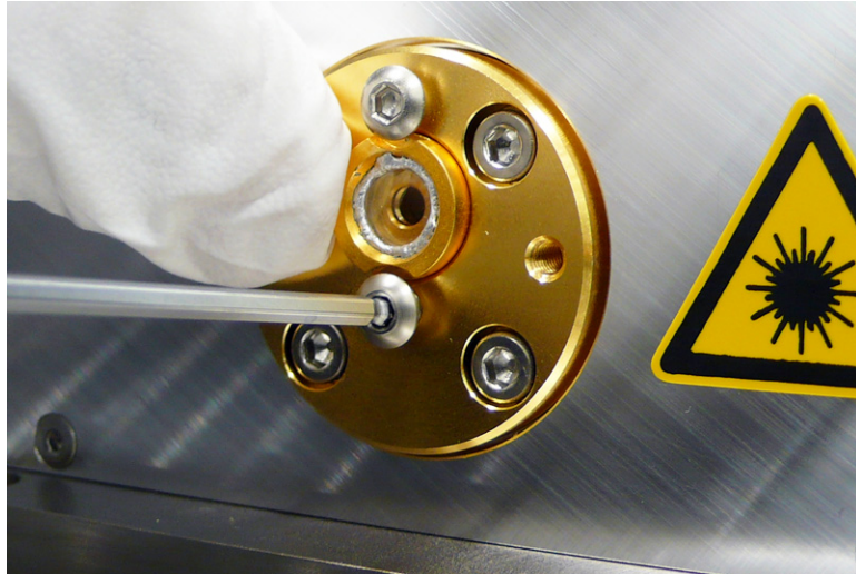
Figure 8-3: Loosen the bottom retaining screw.
