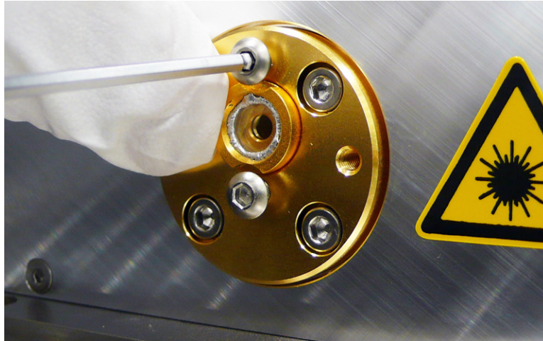
Figure 8-5: Replace the window assembly.
