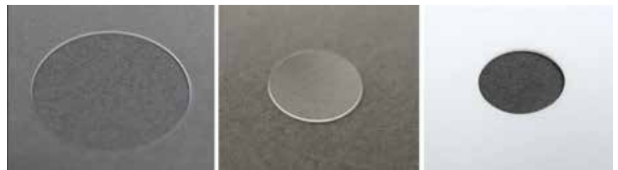
Figure 3. Brittle materials — 200- \mu\text{m} -thick Corning Willow glass (left), 150- \mu\text{m} sapphire (center) and 200- \mu\text{m} alumina (right) — cut with MKS Spectra-Physic IceFyre picosecond hybrid fiber laser.
