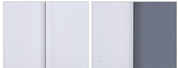
Figure 5. Top down images of sapphire after Bessel processing before (left) and after (right) cleaving.
