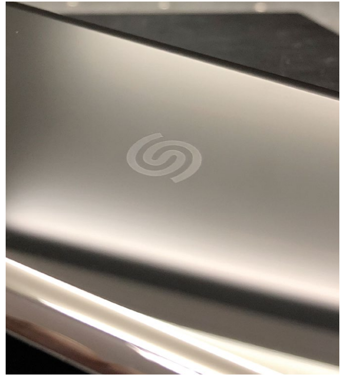
Figure 3: Marking of a logo on a polished ceramic surface
